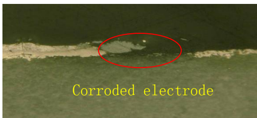
Figure 1 Left top terminal is corroded
